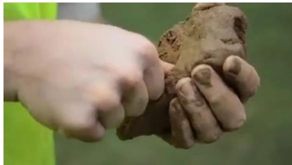
Type C: Easily penetrated by several inches.
