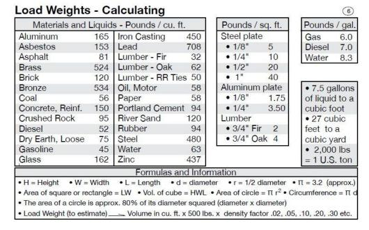
\*THE ACTUAL LOAD MUST NOT EXCEED THE RATED SLING CAPACITY\*
