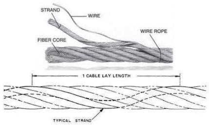
NOTE: Wire Rope Sling inspection shall be conducted on the entire length of the sling including splices, end attachments and fittings for deterioration which would result in loss of original strength.
