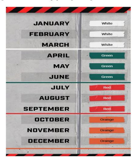
Test verification shall be by means of numeric or color-coded marking tape on the receptacle, cord set or equipment to identify that it has passed the test and to indicate the date (quarter) in accordance with Table above. The year of inspection is identified by a black marker on the tape of the item inspected.
